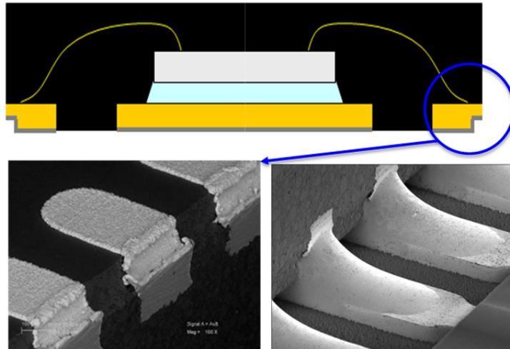
Figure 2: Typical Side solderable swan QFN package
